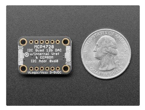
To take things even further, the MCP4728 lets you chose between two sources for your reference voltage: the input voltage that you use to power it on the VCC pin, or an internal 2.048V reference voltage. If you use the internal reference voltage (Vref in DAC speak) you can choose between 1X and 2X gain for the output, allowing your
