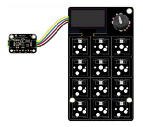
The STEMMA QT port is best for use with I2C devices. You can use any of the Qwiiccompatible I2C breakout boards () available by plugging them into this port and coding them with either the available CircuitPython or Arduino drivers and libraries.
