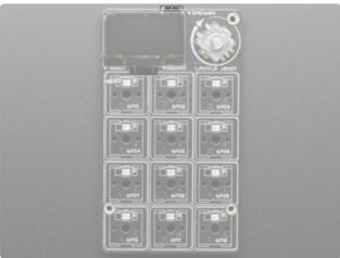
At the top-center of the board, visible from both sides, is the USB Type C connector. This connector is used both for transferring data from your computer (e.g. updating your CircuitPython code.py file, or uploading an Arduino sketch) and powering the board.
