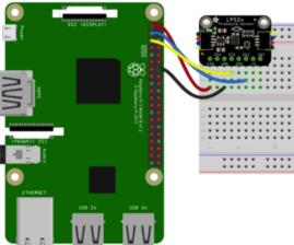
Pi 3V to sensor VCC (red wire)
