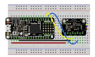
Board 3V to sensor VIN (red wire)
