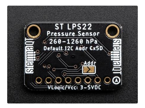
Furthermore, we've included <u>SparkFun Qwiic</u> () compatible <u>STEMMA QT</u> () connectors for the I2C bus so you don't even need to solder! All you need to do is plug in a <u>compatible cable</u> (), wire it up to your device using one of our wiring diagrams and you're ready to write some code to start reporting measurements.
