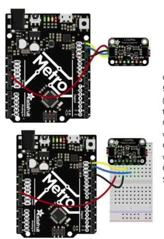
Connect board VIN (red wire) to Arduino 5V if you are running a 5V board Arduino (Uno, etc.). If your board is 3V, connect to that instead. Connect board GND (black wire) to Arduino GND Connect board SCL (yellow wire) to Arduino SCL Connect board SDA (blue wire) to Arduino SDA
