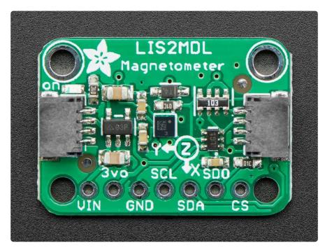
We based this breakout on ST's LIS2MDL, a great general purpose magnetometer. This compact sensor uses I2C to communicate and its very easy to use. Simply download our library and connect the SCL pin to your I2C clock pin, and SDA pin to your I2C data pin and upload our test program to read out magnetic field data. If you'd like, you can also use SPI to receive data (we just happen to prefer I2C here)
