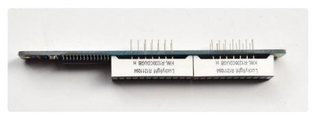
To keep the two bargraphs lined up nicely, you can use a little masking or scotch tape on the bargraph modules, tape them so they are in a straight line. There is a little play during soldering so if you don't do this the two modules may not be in a perfect line.
