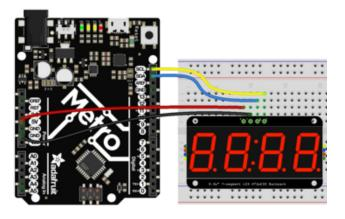
Backpack + (VCC) to microcontroller 5V (if using a board with 5V logic, otherwise use 3V for boards with 3V logic) (red wire) Backpack - (GND) to microcontroller GND
