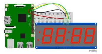
Raspberry Pi 3.3V to 7-Segment Display IO
