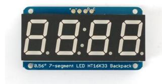
Remove the parts from packaging and place the LED matrix OVER the silkscreen side. DO NOT PUT THE DISPLAY ON UPSIDE DOWN OR IT WONT WORK!! Check the image below to make sure the 'decimal point' dots are on the bottom, matching the silkscreen.
