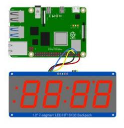
Raspberry Pi 3.3V to STEMMA QT red wire Raspberry Pi GND to STEMMA QT black wire
