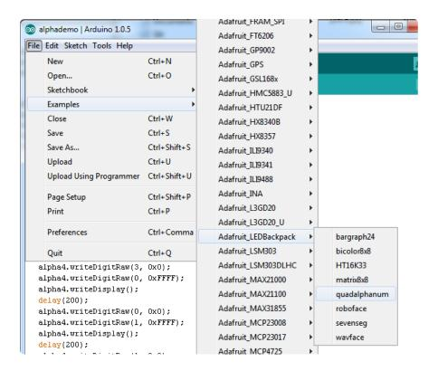
Upload to your Arduino, and open up the Serial console at 9600 baud speed. You'll see each digit light up all the segments, then the display will scroll through the 'font table' showing every character that it knows how to display. Finally, you'll get a notice to start typing into the serial console. Type a message and hit return, you'll see it scroll onto the display!
