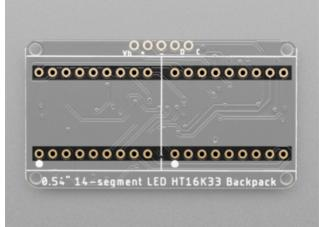
These two rows of through-hole pads are for soldering the alphanumeric LED displays onto the backpack. See the Assembly page () for details on attaching the displays properly.
