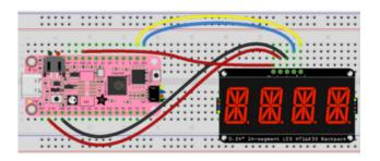
Board 5V to backpack Vio (red wire connected along the bottom of the Feather)
