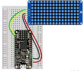
Microcontroller 3V to LED Matrix VIN
