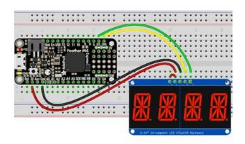
Microcontroller 3V to AlphaNumeric Display I2C VIN
