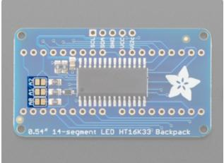
On the back of the board are three address jumpers, labeled AO, A1, and A2. These jumpers allow you to chain up to 8 of these boards on the same pair of I2C clock and data pins. To do so, you solder the jumpers "closed" in various combinations by connecting the two pads.
