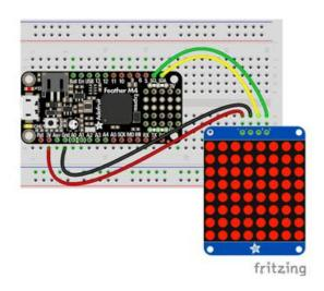
Microcontroller 3V to LED Matrix VIN
