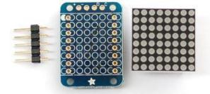
When you buy a pack from Adafruit, it comes with the fully tested and assembled backpack as well as a 8x8 matrix in one of the colors we provide (say, red, yellow or green). You'll need to solder the matrix onto the backpack but its an easy task.
