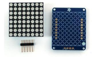
When you buy a pack from Adafruit, it comes with the fully tested and assembled backpack as well as a 8x8 matrix in one of the colors we provide (say, red, yellow or green). You'll need to solder the matrix onto the backpack but its an easy task.
