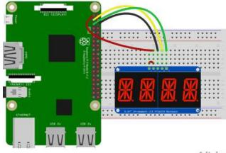
Raspberry Pi 3.3V to AlphaNumeric Display I2C VIN
