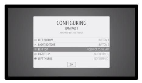
Although the Joy Bonnet has an analog stick, the software installed above makes this act like a digital 4-way stick emitting key presses. This is on purpose and by design, as Retropie on a single-stick controller like this expects digital inputs.
