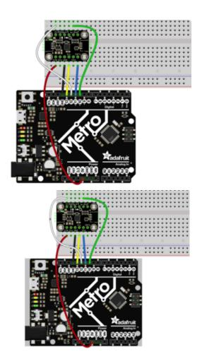
Connect Vin to the power supply, 3V or 5V is fine. Use the same voltage that the microcontroller uses
