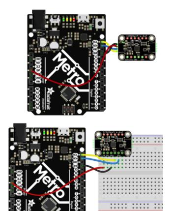
Connect board VIN (red wire) to Arduino 5V if you are running a 5V board Arduino (Uno, etc.). If your board is 3V, connect to that instead.
