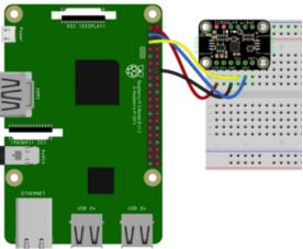
Pi 3V to sensor VCC (red wire)
