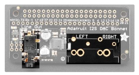
There's also a breakout slot for soldering in dual/stereo RCA jacks, not included with the bonnet.
