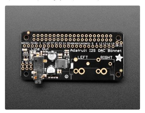
This Bonnet uses I2S a digital sound standard, so you get really crisp audio. The digital data goes right into the amplifier so there's no static like you hear from the onboard headphone jack. And it's super easy to get started. Just plug in any line level output into powered speakers or audio system. You can plug in headphones but you'll get some distortion - so its best used into something that is expecting line level out
