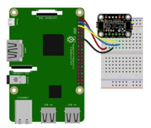
Pi 3V to sensor VCC (red wire)
