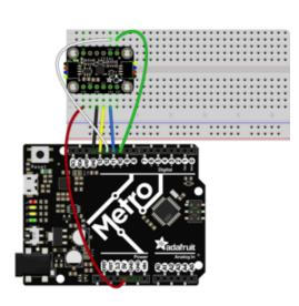
Connect Vin to the power supply, 3V or 5V is fine. Use the same voltage that the microcontroller logic is based off of Connect GND to common power/data ground
