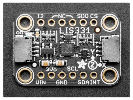
It's not hard to find an accelerometer that can measure accelerations up to 16g, but if you need an accelerometer that can measure even larger amounts of acceleration, your options narrow (The ICM20649 () is a great sensor and can measure up to  $\pm 30g$ ).
