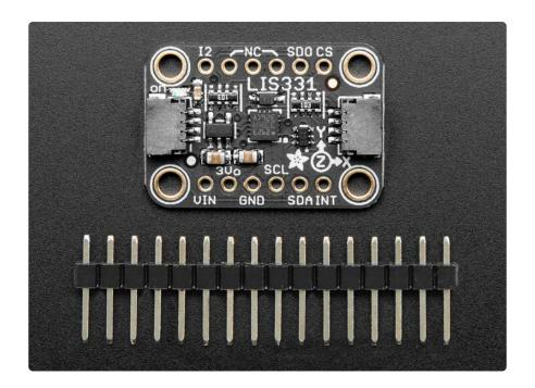
In addition to their substantial measurement capability, the LIS331s have built in and c onfigurable high-pass and low-pass filters to adjust the readings to your application. Adjustable data rates also allow you to adjust how frequently to take measurements depending on your power budget, and SPI and I2C interfaces give them flexibility to allow them to be used in a range of applications.
