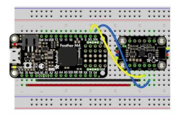
Board 3V to sensor VIN (red wire)
