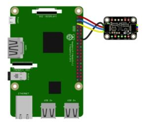
Pi 3V to sensor VCC (red wire)
