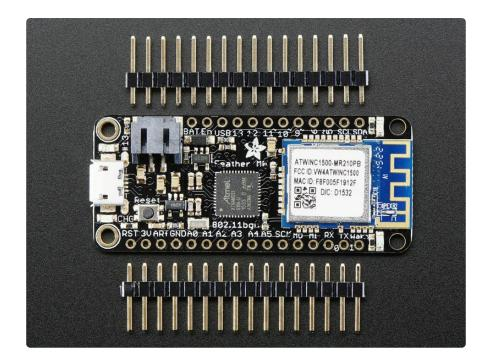
Comes fully assembled and tested, with a USB bootloader that lets you quickly use it with the Arduino IDE. We also toss in some header so you can solder it in and plug into a solderless breadboard. <u>Lipoly battery</u> () and <u>MicroUSB cable</u> () not included (but we do have lots of options in the shop if you'd like!)
