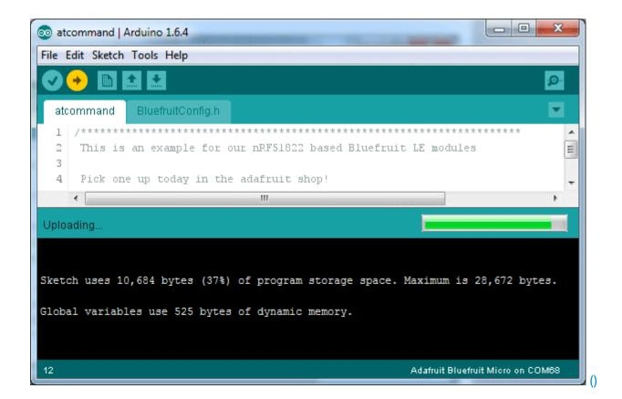
Don't click the reset button before uploading, unlike other bootloaders you want this one to run at the time Arduino is trying to upload
