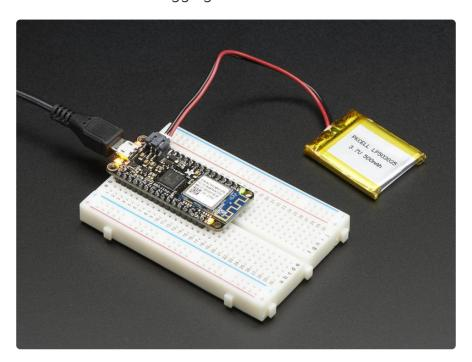
To make it easy to use for portable projects, we added a connector for any of our 3.7V Lithium polymer batteries and built in battery charging. You don't need to use a battery, it will run just fine straight from the micro USB connector. But, if you do have a
