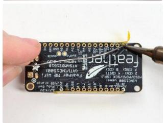
After flipping over, solder one or two points on each strip, to 'tack' the header in place
