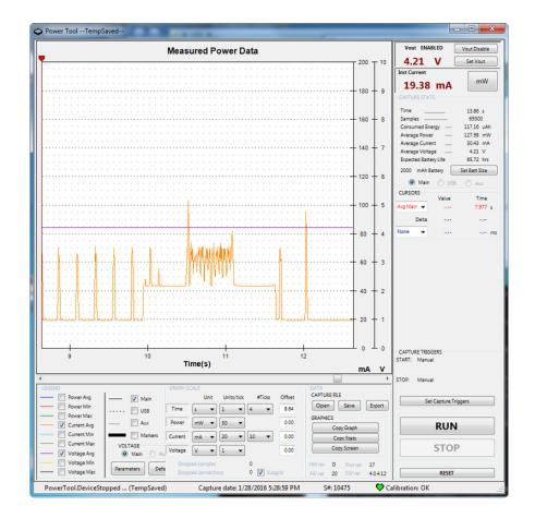
Note that the quiescent current drops from 40mA to 20mA and of that 20mA, about ~12mA is the ATmega32u4. Like we said, the best way to really reduce power for long-term usage is to completely turn off the module with KEY
