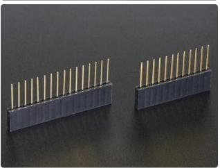
Finally, there's the "Stacking Header" option. This one is sort of the best-of-bothworlds. You get the ability to plug into a solderless breadboard and plug a featherwing on top. But its a little bulky
