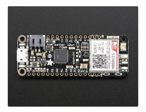
Since you'll be taking this on the road, we added a connector for any of our 3.7V Lithium polymer batteries and built in battery charging. A 500mAh+ Lipoly battery is required for use, it keeps the cellular module happy during the high current spikes. Plug the Feather into microUSB to charge at 500mA.
