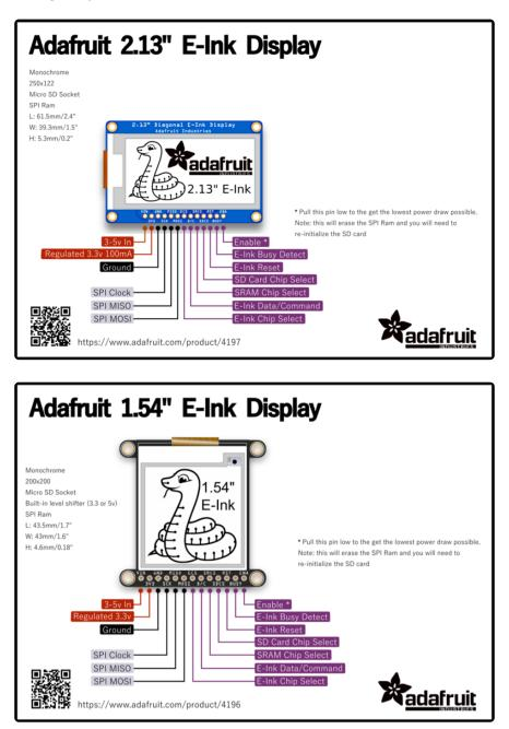
The pin outs are identical for the 1.54", 2.13" and 2.7" E-Ink display!
