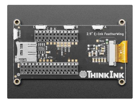
This e-Paper display uses SPI to receive image data. Since the display is SPI, it was easy to add two more SPI devices to share the bus - an SPI SRAM chip and SPI-driven SD card holder. There's quite a few pins and a variety of possible combinations for control depending on your needs.
