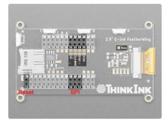
The FeatherWing uses SPI and some control pins for reading/writing data from the SD and then sending data to the E-Ink display
