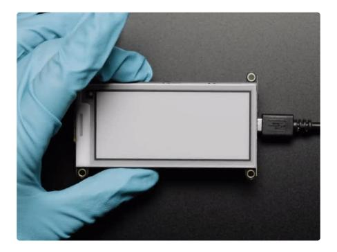
Easy e-paper comes to your Feather with this breakout that's designed to make it a breeze to add a monochrome elnk display. Chances are you've seen one of those new-fangled 'e-readers' like the Kindle or Nook. They have gigantic electronic paper 'static' displays - that means the image stays on the display even when power is completely disconnected. The image is also high contrast and very daylight readable. It really does look just like printed paper!
