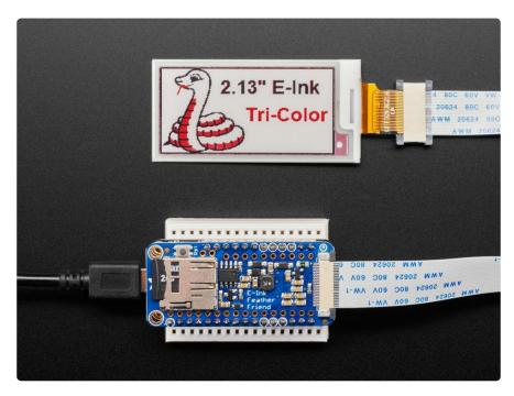
On the Breakouts and Shields, We even tossed on a MicroSD socket so you can store images, text files, whatever you like to display. Everything is 3 or 5V logic safe so you can use it with any and all microcontrollers.
