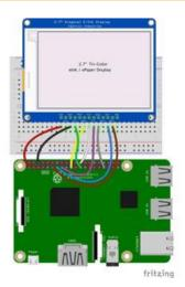
Raspberry Pi 3.3 to display VIN Raspberry Pi GND to display GND Raspberry Pi SCLK to display SCK Raspberry Pi MOSI to display MOSI Raspberry Pi GPIO CE0 to display ECS Raspberry Pi GPIO 22 to display D/C Raspberry Pi GPIO 27 to display RST Raspberry Pi GPIO 17 to display BUSY
