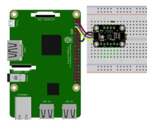
Connect board Vcc (long red wire) to Pi 3.3V
