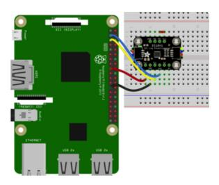
Connect board Vcc (long red wire) to Pi 3.3V
