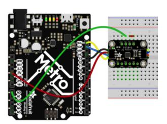
Connect board VIN (red wire) to Metro 5V if you are running a 5V board Arduino (Uno, etc.). If your board is 3V, connect to that instead.
