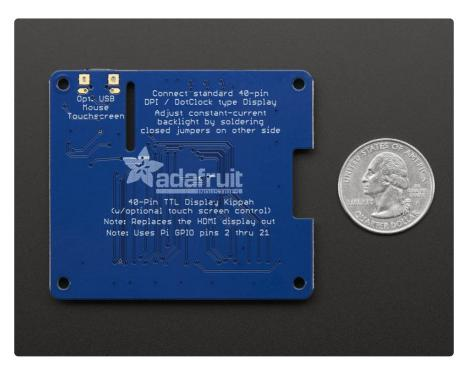
Comes as one fully assembled and tested DPI Kippah circuit board. You may need a soldering iron to adjust the backlight by soldering closed a PCB jumper (check the tutorial on this). TFT display (), USB micro-B cable (http://adafru.it/592), FPC extension cable (), bent wire stand (), and Raspberry Pi not included (but we do carry them in the shop!)
