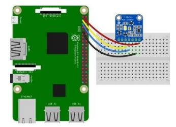
Pi 3V3 to sensor VIN Pi GND to sensor GND
