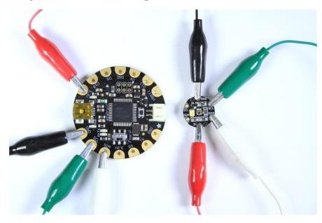
Both color sensors come with all surface mount components pre-soldered. The breakout-board version comes with an optional header for breadboard use. Soldering the header is a simple process:
