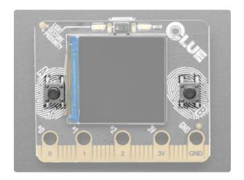
A and B buttons - The CLUE has two user-programmable buttons on the front, labeled A and B. Use them as inputs to control your code. These are unconnected when not pressed, and connected to GND when pressed, so they read LOW. Set the pins to use an internal pull-UP when reading these pins so they will read HIGH when not pressed. Buttons can be addressed in CircuitPython using board.BUTTON\_A and board.BUTTON\_B, and in Arduino as D5 (left button) and D11 (right button).
