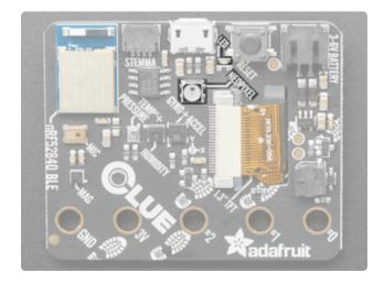
NeoPixel - The addressable RGB NeoPixel LED is used as a status LED by the bootloader and CircuitPython, but is also controllable using code. Control it using board.NEOPIXEL in CircuitPython and D18 in Arduino.
