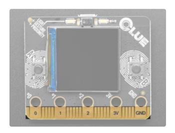
Micro:Bit compatible edge connector - This is the Micro:Bit compatible edge connector, used to break out all of the other features of this microcontroller.
