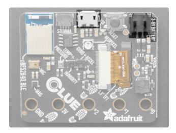
USB Micro - This USB port is used for programming and/or powering the CLUE. It is a standard USB Micro connector.
