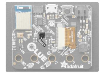
Humidity: SHT30 - This sensor has an excellent  $\pm 2\%$  relative humidity and  $\pm 0.5$ °C accuracy for most uses. Sensor is I2C on standard pins on address 0x44.
