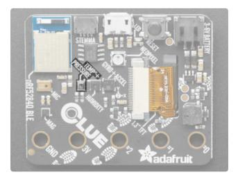
Temp + Pressure: BMP280 - This sensor is a precision sensing solution for measuring barometric pressure with ±1 hPa absolute accuraccy, and temperature with ±1.0°C accuracy. Because pressure changes with altitude, and the pressure measurements are so good, you can also use it as an altimeter with ±1 meter accuracy. It has a a low altitude noise of 0.25m and a fast conversion time. Sensor is I2C on standard pins on address 0x77.
