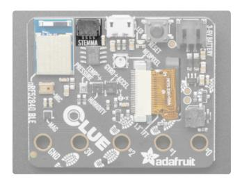
Qwiic / STEMMA QT connector - Use to add more sensors, motor controllers, or displays over I2C. You can plug in GROVE I2C sensors by using an adapter cable (). In CircuitPython, you can use the STEMMA connector
