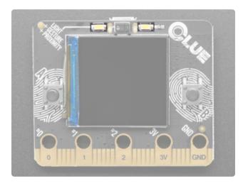
Bright white LEDs - On the front of the board are two bright white LEDs for illumination and color sensing. Control them in CircuitPython using board.WHITE\_LEDS, and in Arduino using D43.
