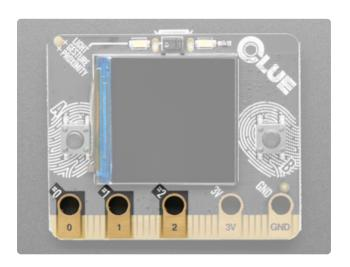
Pads 0, 1 and 2 - These pads are used for connecting external sensors etc, typically using alligator clips. They also work as inputs using capacitive touch. In CircuitPython they are board.D0, board.D1, and board.D2. In Arduino, they are D0, D1 and D2.
