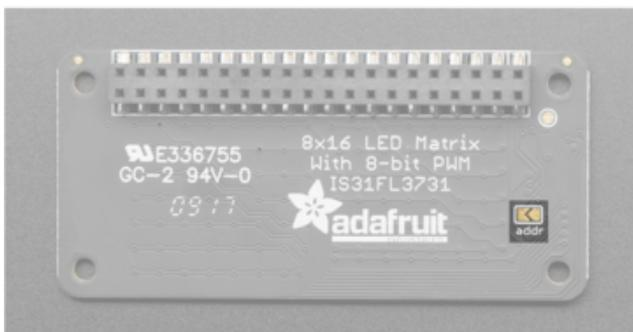
The default I2C address for the Bonnet is `0x74`. Solder this jumper closed to change it to `0x70` to avoid I2C address conflicts, if needed.
