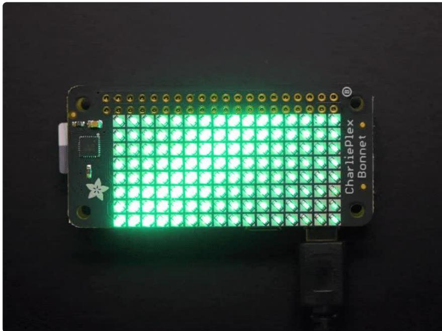
You won't be able to look away from the mesmerizing patterns created by this Adafruit CharliePlex LED Matrix Display Bonnet. This 16x8 LED display can be placed atop any Raspberry Pi computer with a 2x20 connector, for a beautiful, bright grid of 128 CharliePlexed LEDs. It even comes with a built-in CharliePlex driver that is run over I2C.
