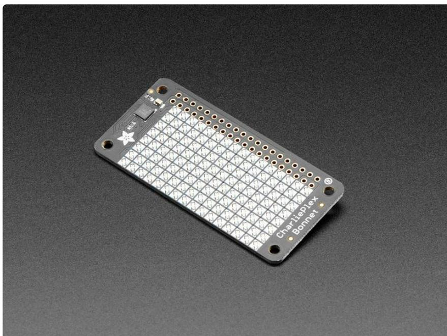
What is particularly nice about this Bonnet is the I2C LED driver chip has the ability to PWM each individual LED in a 16x8 grid so you can have beautiful LED lighting effects, without a lot of pin twiddling. Simply tell the chip which LED on the grid you want lit, and what brightness and it's all taken care of for you. You get 8-bit (256 level) dimming for each individual LED.
