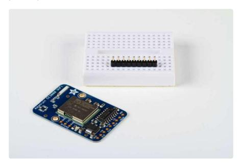
Set the breakout board over the pins, and carefully solder each pin (see our <u>Guide To</u> Excellent Soldering () for instructions and tips on getting the best results).
