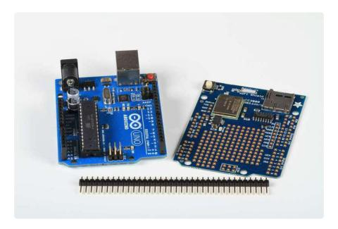
The CC3000 Shield ships with a strip of header pins.
