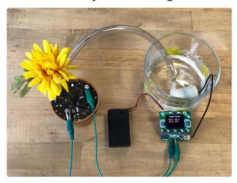
It's easy to use the Adafruit Bonsai Buckaroo with CircuitPython. This example uses the Adafruit CircuitPython CLUE () library to display soil moisture level and the status of the pump motor on the CLUE display. Connect your Bonsai Buckaroo to your CLUE, and connect the motor and plant to the Bonsai Buckaroo, and you're on your way to automatic plant care. Let's take a look!
