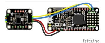
Board 3V to sensor VIN (red wire for STEMMA QT) Board GND to sensor GND (black wire for STEMMA QT) Board SCL to sensor SCL (yellow wire for STEMMA QT) Board SDA to sensor SDA (blue wire for STEMMA QT)
