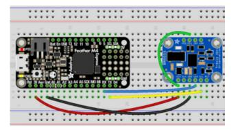
Board 3V to sensor VIN Board GND to sensor GND Board TX to sensor SCL Board RX to sensor SDA sensor PS1 to sensor VIN
