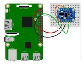
Pi 3V3 to sensor VIN Pi GND to sensor GND Pi TXD to sensor SCL Pi RXD to sensor SDA sensor PS1 to sensor VIN
