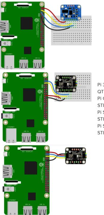
Pi 3V3 to sensor VIN (red wire for STEMMA QT) Pi GND to sensor GND (black wire for STEMMA QT) Pi SCL to sensor SCL (yellow wire for STEMMA QT) Pi SDA to sensor SDA (blue wire for STEMMA QT)
