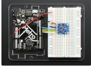
Connect Vin to the power supply, 3V or 5V is fine. Use the same voltage that the microcontroller logic is based off of. For most Arduinos, that is 5V Connect GND to common power/data
