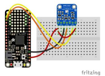
And an example of a Feather M0 wired with hardware SPI:
