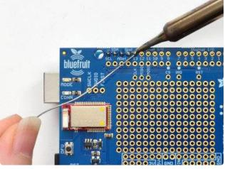
Solder in all the header on the top strips
