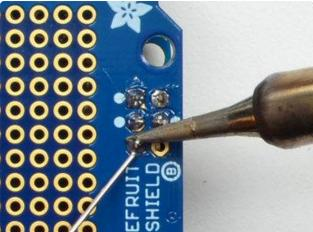
Don't forget the 6-pin socket!
