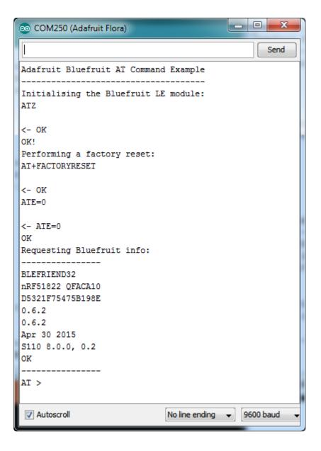
To send an AT command to the Bluefruit LE module, enter the command in the textbox at the top of the Serial Monitor and click the Send button:
