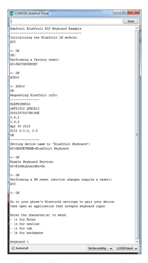
To send keyboard data, type anything into the textbox at the top of the Serial Monitor and click the Send button.
