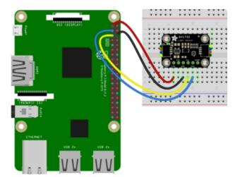
Pi 3V to sensor VCC (red wire) Pi GND to sensor GND (black wire) Pi SCL to sensor SCL (yellow wire) Pi SDA to sensor SDA (blue wire)
