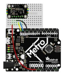
Connect board VIN (red wire) to Arduino 5V if you are running a 5V board Arduino (Uno, etc.). If your board is 3V, connect to that instead. Connect board GND (black wire) to Arduino GND Connect board SCL (yellow wire) to Arduino SCL Connect board SDA (blue wire) to Arduino SDA
