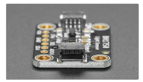
To make things easier and a bit more flexible, we've also included <u>SparkFun Qwiic</u> () compatible <u>STEMMA QT</u> () connectors for the I2C bus so you don't even need to solder! Just plug in a compatible cable and attach it to your MCU of choice and you're ready to load up some software and measure some light. To help with the software
