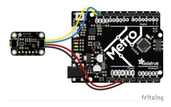
Connect board VIN (red wire) to Arduino 5V if you are running a 5V board Arduino (Uno, etc.). If your board is 3V, connect to that instead. Connect board GND (black wire) to Arduino GND Connect board SCL (yellow wire) to Arduino SCL Connect board SDA (blue wire) to Arduino SDA
