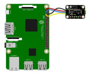
Pi 3V to sensor VCC (red wire) Pi GND to sensor GND (black wire) Pi SCL to sensor SCL (yellow wire) Pi SDA to sensor SDA (blue wire)
