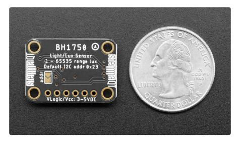
The BH1750 provides 16-bit light measurements in lux, the SI unit for measuring light making it easy to compare against other values like references and measurements from other sensors. Able to measure from 0 to 65K+ lux, the BH1750. With some
