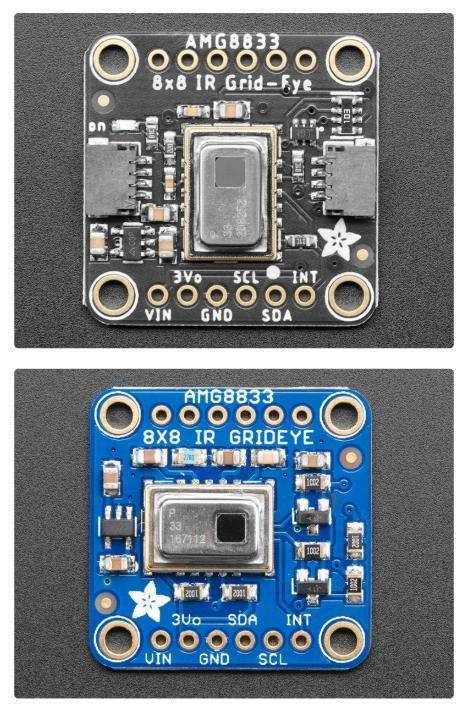
This camera has 4 mounting holes, and two header strips. Only the bottom strip is connected to the sensor. The top set of breakouts is there for mechanical stability only!
