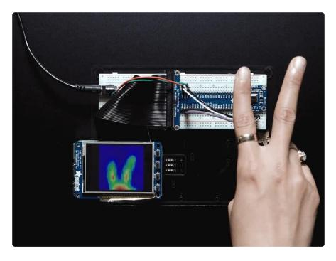
The AMG8833 is the next generation of 8x8 thermal IR sensors from Panasonic, and offers higher performance than it's predecessor the AMG8831. The sensor only supports I2C, and has a configurable interrupt pin that can fire when any individual pixel goes above or below a thresholds that you set.
