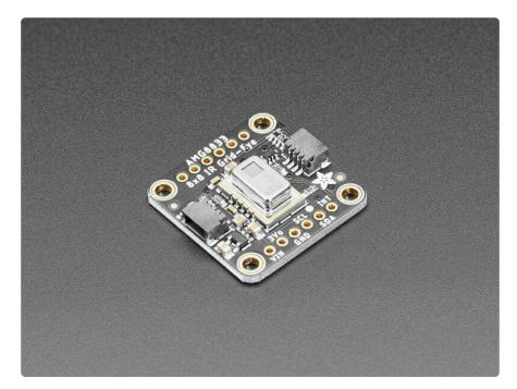
This part will measure temperatures ranging from 0°C to 80°C (32°F to 176°F) with an accuracy of +- 2.5°C (4.5°F). It can detect a human from a distance of up to 7 meters (23) feet. With a maximum frame rate of 10Hz, It's perfect for creating your own human
