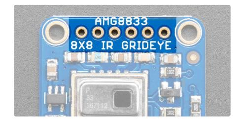
The 6 holes at the top of the board are provided for stability and are not connected to anything. Use these if you want your sensor to sit nice and flat on a breadboard or Perma-Proto.
