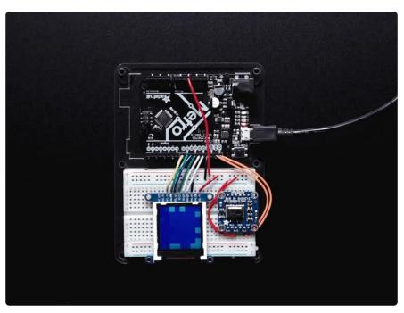
Add heat-vision to your project and with an Adafruit AMG8833 Grid-EYE Breakout! This sensor from Panasonic is an 8x8 array of IR thermal sensors. When connected to your microcontroller (or raspberry Pi) it will return an array of 64 individual infrared temperature readings over I2C. It's like those fancy thermal cameras, but compact and simple enough for easy integration.
