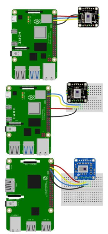
Pi 3V3 to sensor VIN (red wire on STEMMA QT version) Pi GND to sensor GND (black wire on STEMMA QT version) Pi SCL to sensor SCL (yellow wire on STEMMA QT version) Pi SDA to sensor SDA (blue wire on STEMMA QT version)
