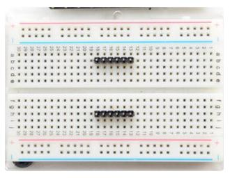
Prepare the header strips: Cut the strips to length if necessary. It will be easier to solder if you insert it into a breadboard - long pins down
