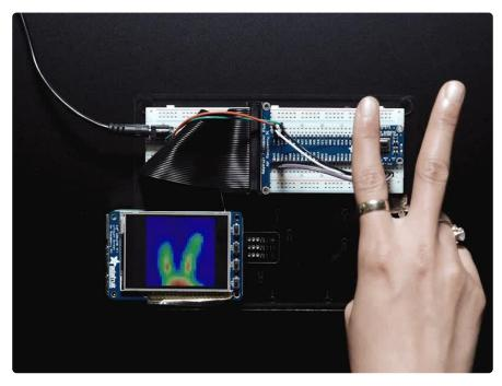
The Raspberry Pi also has an i2c interface, and even better has processing capability to interpolate and filter the sensor output. By adding processing power, you can 'turn' the 8x8 output into what appears to be a higher-resolution display.
