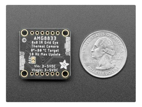
Should you wish to avoid soldering, we now also include our <u>Stemma QT</u> () connector s (<u>SparkFun Qwiic</u> () compatible). Using these handy connectors you can simply plug in the sensor, no soldering required! <u>QT Cable is not included, but we have a variety</u> in the shop ().
