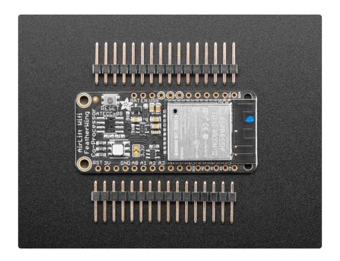
We placed an ESP32 module on a FeatherWing with a separate 3.3V regulator, and a tri-state chip for MOSI so you can share the SPI bus with other 'Wing. Comes fully assembled and tested, pre-programmed with ESP32 SPI WiFi co-processor firmware that you can use in CircuitPython to use this into WiFi co-processor over SPI + 2 pins (). We also toss in some header so you can solder it in and plug into a doubler, but you can also pick up a set of stacking headers to stack above/below your Feather.
