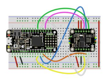
BNO085 Vin to 3V on the Feather M4 BNO085 GND to common power/data ground
