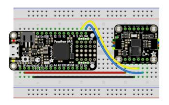
Board 3V to sensor VIN (red wire)
