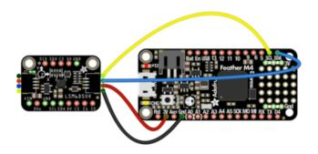
Board 3V to sensor VIN (red wire)
