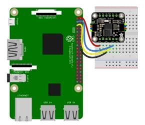
Pi 3V to sensor VCC (red wire)
