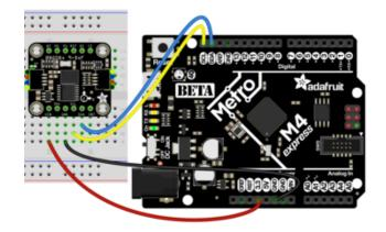
Connect board VIN (red wire) to Board 3V Connect board GND (black wire) to Board GND
