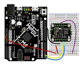
BNO085 Vin to the power supply, using the same logic level as your microcontroller. For the Metro M4 shown that is 3.3V, however check your board's documentation to be sure BNO085 GND to board GND BNO085 SCL to board TX BNO085 SDA to board RX BNO085 P1 to Board Power supply
