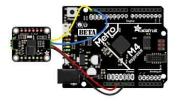
Connect board VIN (red wire) to Board 3V Connect board GND (black wire) to Board GND
