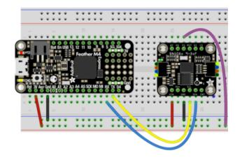
Board 3V to sensor VIN (red wire)
