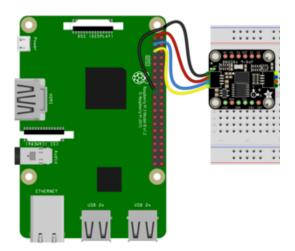
Pi 3V to sensor VCC (red wire)
