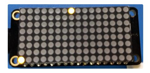
You can also make the entire display blink at 3 different rates using the blink\_rate property, which has a value 0 to 3:
