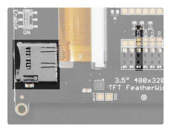
The SD Card also has a Chip Select line, labeled SD. This pin can theoretically be changed by cutting the jumper trance and soldering a small wire from the right-hand pad to the pin you'd like to use.
