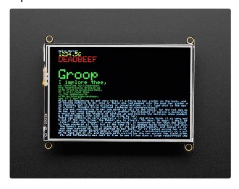
The TFT FeatherWing is basically a combination of our 3.5" TFT Breakout () with the 5 TMPE610 resistive touch-screen breakout attached (http://adafru.it/1571).
