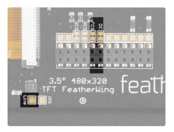
In addition, for the TFT display there is are D/C (Data/Command) and CS (Chip Select) pins. These are used to select the display and tell it what kind of data is being sent. These pins can theoretically be changed by cutting the jumper trace and soldering a small wire from the farther-from-the-socket-header pad to the pin you'd like to use.
