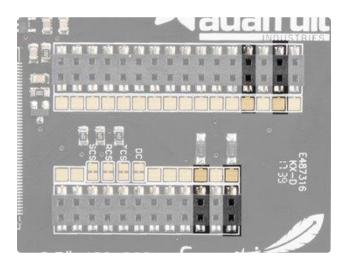
The 3.5" TFT FeatherWing has a really beefy backlight, and we don't want to overwhem the 3.3V regulator on the Feather so we use two Schottkey diodes to take the higher of VBAT and VUSB to feed into the backlight boost converter.
