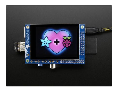
Uses the hardware I2C Pins (SDA & SCL), SPI pins (SCK, MOSI, MISO, CEO) as well as GPIO #25 and #24. All other GPIO are unused. Since we had a tiny bit of space, there's 4 spots for optional slim tactile switches wired to four GPIOs, that you can use if you want to make a basic user interface. For example, you can use one as a power on/off button. See below for the link to get the optional tact switches, they're not included.
