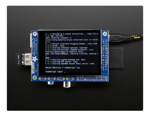
The screen is the same size as the resistive type so you can use this with the PiTFT PiBow or any other enclosure you may already have. We also use the same SDL device and signals so PyGame and X11 based programs can be swapped in with no changes in code.
