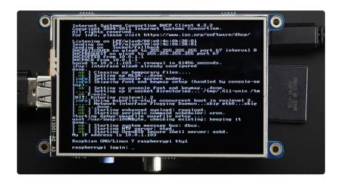
One fun thing you can do with the display is have it as your main console instead of the HDMI/TV output. Even though it is small, with a good font you can get 20 x 40 of text. For more details, check out https://github.com/notro/fbtft/wiki/Boot-console ()
