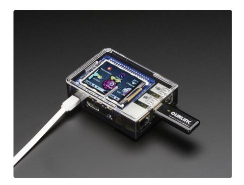
This design uses the hardware SPI pins (SCK, MOSI, MISO, CE0, CE1) as well as GPIO #25. All other GPIO are unused. Since we had a tiny bit of space, there's 4 flat tactile switches wired to four GPIOs, that you can use if you want to make a basic user interface. For example, you can use one as a power on/off button.
