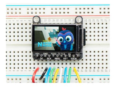
To make new bitmaps, make sure they are less than 240 by 135 pixels and save them in 24-bit BMP format! They must be in 24-bit format, even if they are not 24-bit color as that is the easiest format for the Arduino. You can rotate images using the setRotati on() procedure
