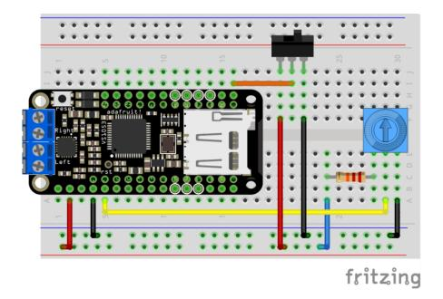
Power up your radio and flip the switch to the power side to turn it on. Try flipping the switch once the radio starts playing to see if it shuts off.
