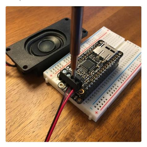
Tighten the screws and we are ready to load some music onto the SD card.
