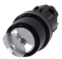
RONIS key-operated switch, 22 mm, round, plastic, lock number SB30, with 2 keys, 2 switch positions O-I, latching, actuating angle 90°, 10:30h/13:30h, key removal O+I, possible special locks: SB31, 421, 455, with laser labeling, upper case and lower case, always upper case at beginning of line
