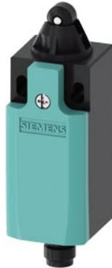
Position switch Plastic 31 mm according to EN 50047 Increased corrosion protection with M12 connector plug, 4-pole 1 NO/1 NC quick action contacts Roller plunger with plastic roller 10 mm functional at -40 °C Shock and vibration test according to EN 61373, Category 1B
