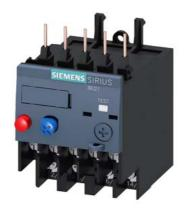
Overload relay 0.90...1.25 A Thermal For motor protection Size S00, Class 10 Contactor mounting Main circuit: Ring cable lug Auxiliary circuit: ring cable lug Manual-Automatic-Reset
