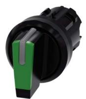
Selector switch, illuminable, 22 mm, round, plastic, green, selector switch, short, 3 switch positions I>O<II, momentary contact type, actuating angle 2x45°, 10:30h/12h/13:30h Z=50-unit packaging
