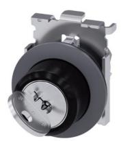
RONIS key-operated switch, 30 mm, round, Metal, matte, front ring for flush installation, lock number SB30, with 2 keys, 2 switch positions O-I, latching, actuating angle 90°, 10:30h/13:30h, key removal O+I, possible special locks: SB31, 421, 455, with laser labeling, upper case and lower case, always upper case at beginning of line
