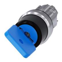
Key-operated switch O.M.R, 22 mm, round, metal, shiny, lock number 73038, blue, with 2 keys, 2 switch positions O-I, latching, actuating angle 90°, 10:30h/13:30h, key removal I, with laser labeling, upper case and lower case, always upper case at beginning of line
