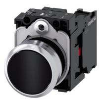
Pushbutton, 22 mm, round, metal, shiny, black, pushbutton, flat, momentary contact type, with holder, 1 NC, screw terminal, with laser labeling, symbol number according to, ISO 7000 or IEC 60417
