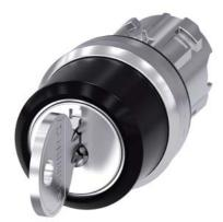
RONIS key-operated switch, 22 mm, round, metal, shiny, lock number SB30, with 2 keys, 3 switch positions I-O<II, left latching, right momentary contact type, actuating angle 2x45°, 10:30h/12h/13:30h, key removal I, possible special locks: SB31, 421, 455, with laser labeling, upper case
