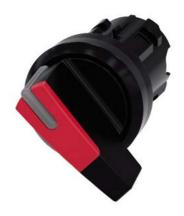
Selector switch, illuminable, 22 mm, round, plastic, red, selector switch, long, 2 switch positions O-I, latching, actuating angle 90°, 10:30h/13:30h, with laser labeling, inscription or symbol Customer-specific selection with SIRIUS ACT configurator (CIN)
