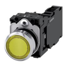
Illuminated pushbutton, 22 mm, round, Metal, shiny, yellow, pushbutton, flat, momentary contact type, with holder, 1 NO+1 NC, LED module with integrated LED 230 V AC, screw terminal, with laser labeling, inscription or symbol Customer-specific selection with SIRIUS ACT configurator (CIN)
