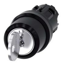
RONIS key-operated switch, 22 mm, round, plastic, lock number SB30, with 2 keys, 3 switch positions I>O<II, momentary contact on the left, latching on the right, actuating angle 2x45°, 10:30h/12h/13:30h, Key removal II, possible special locks: SB31, 421, 455, with laser labeling, upper case and lower case, always upper case at beginning of line
