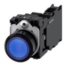
Illuminated pushbutton, 22 mm, round, plastic, blue, pushbutton, flat, momentary contact type, with holder, 1 NO+1 NC, LED module with integrated LED 110 V AC, spring-type terminal, with laser labeling, lower case
