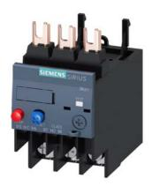
Overload relay 17...22 A Thermal For motor protection Size S0, Class 10 Contactor mounting Main circuit: Ring cable lug Auxiliary circuit: ring cable lug Manual-Automatic-Reset
