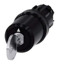
Key-operated switch BKS, 22 mm, round, plastic, lock number S1, with 2 keys, 3 switch positions I-O<II, left latching, right momentary contact type, actuating angle 2x45°, 10:30h/12h/13:30h, key removal O+I, with laser labeling, upper case and lower case, always upper case at beginning of line
