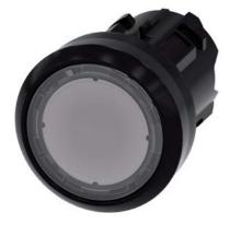
Illuminated pushbutton, 22 mm, round, plastic, clear, pushbutton, flat, latching, Push-to-release mechanism, with laser labeling, symbol number according to, ISO 7000 or IEC 60417
