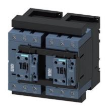
Reversing contactor assembly, AC-3, 55 kW 400 V, 20-33 V AC/DC 3-pole, Size S3 screw terminal electrical and mechanical interlock 2 NO and varistor integrated
