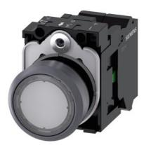
Illuminated pushbutton, 22 mm, round, plastic with metal front ring, clear, pushbutton, flat, momentary contact type, with holder, 1NO, LED module with integrated LED 24 V AC/DC, spring-type terminal, with laser labeling, lower case
